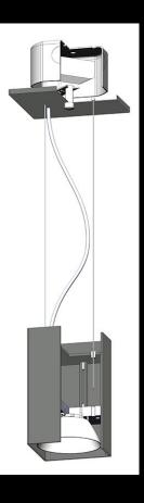
driver mounted in J-box: constant current, field maintainable, universal input (120-277v), 0-10v controllable to 5% dimming \*\*2-1/8" deep J-box required (by other)
